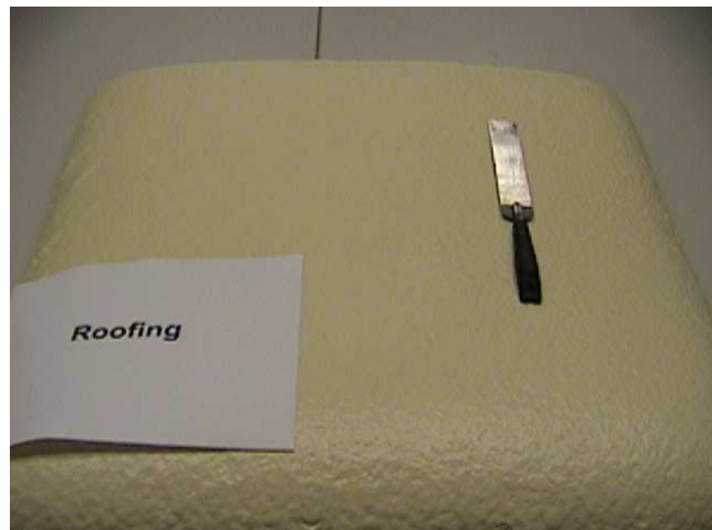
Figure 3. The appearance of 245fa/water co-blown spray roof foam
